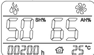
If humidity setting is greater than ambient humidity, the unit will stop working after started 1 minute.
